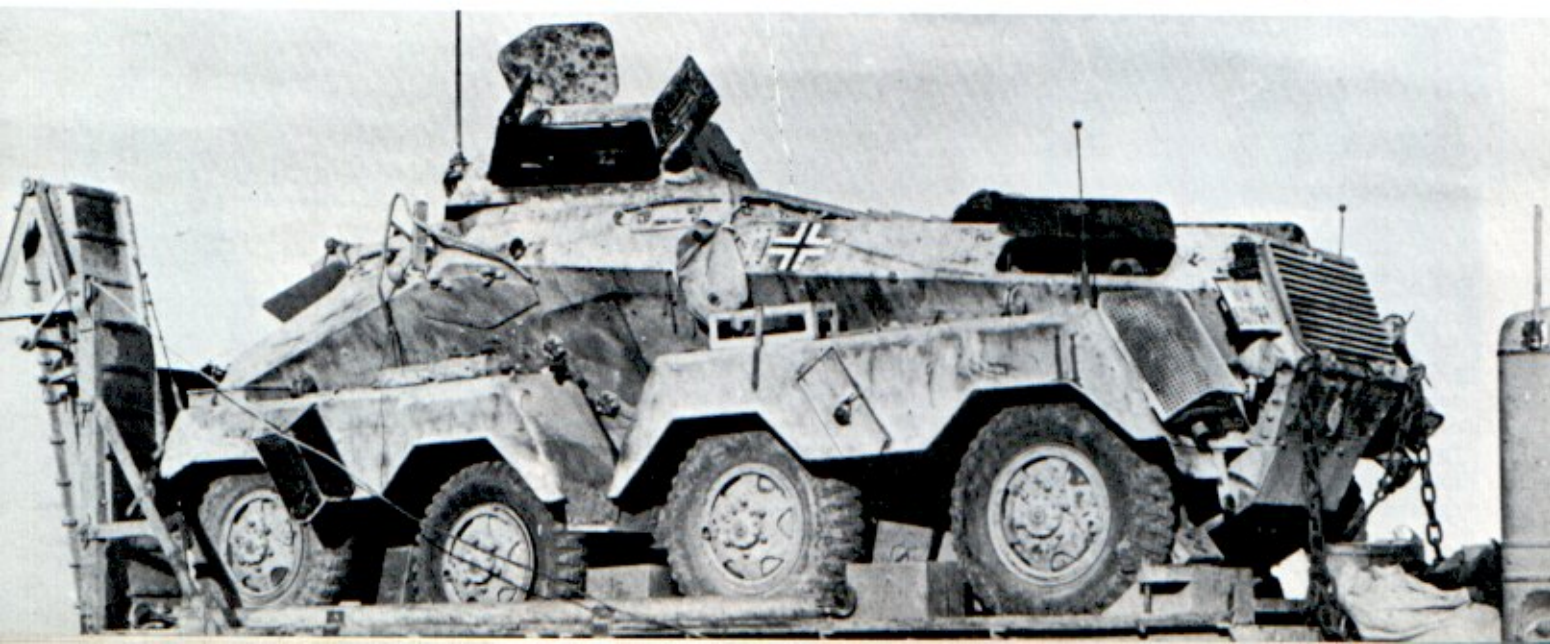
This captured SdKfz 231 [8 rad] armored car, although damaged by an internal fire, shows a badly deteriorated coat of camouflage paint. Note the stains from oil and grease, and the chalky appearance of the paint coating.
