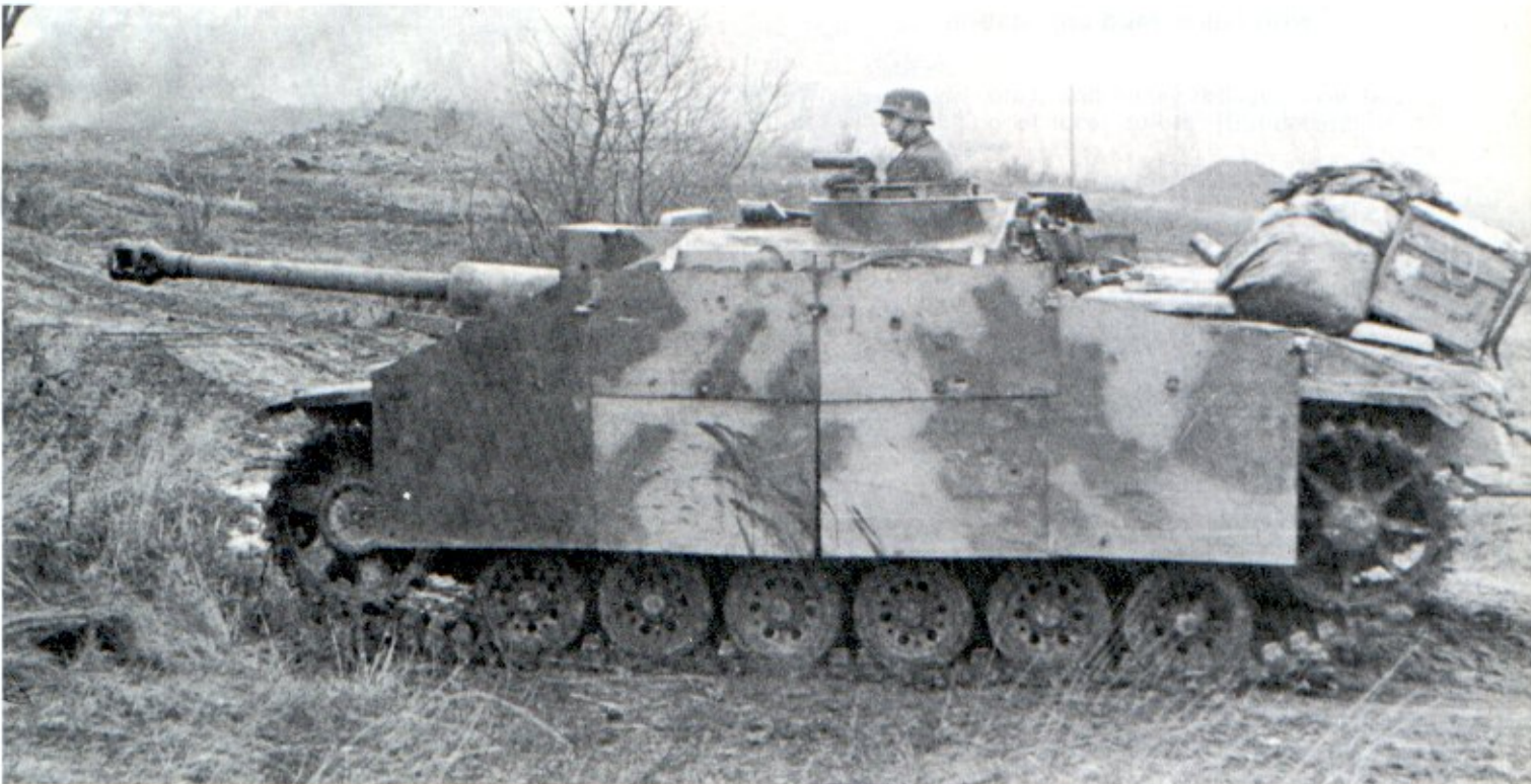
This StuG III ausf G in Russia is painted in a sprayed scheme of red brown over dark yellow. Binocular spotting telescopes protrude from the cupola hatch. The wheels and tracks are covered with mud. Note the sections in the side skirts of this version. [Bundesarchiv]
