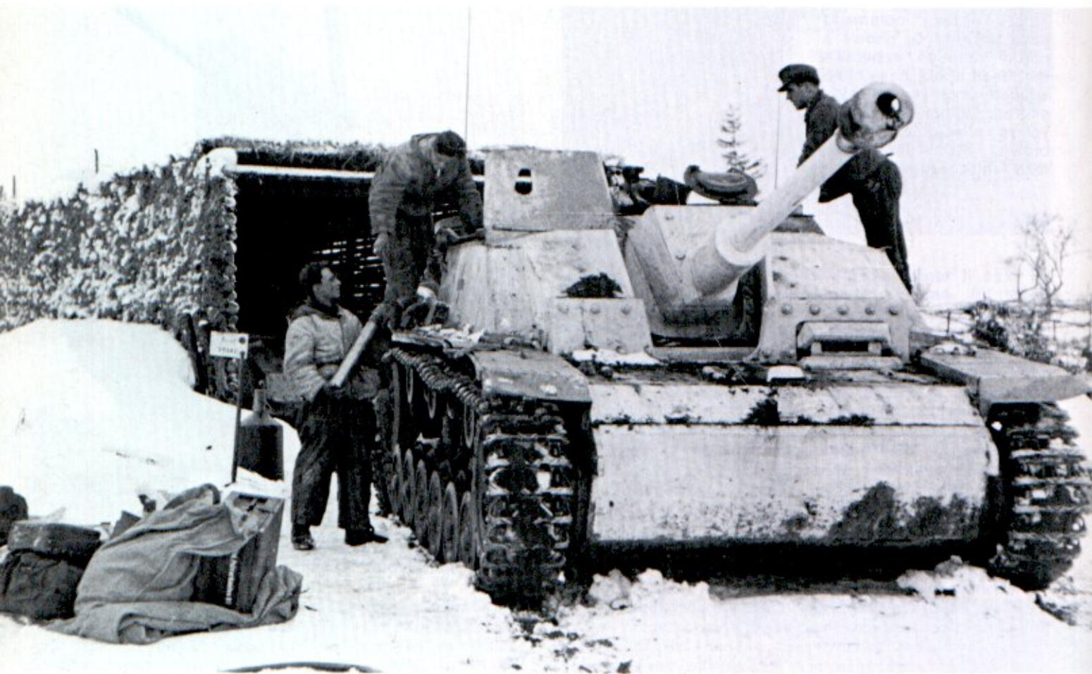
The white camouflage on the StuG III ausf G is badly deteriorated. In particular note the large camouflage "blind" behind the vehicle. The StuG III was normally parked in the "blind" for better concealment. [Bundesarchiv]
