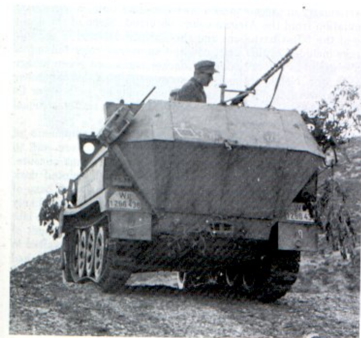
This SdKfz 251/7 engineers' vehicle again shows the application of dark yellow over the dark gray base. This was not confined to Africa but was done there first, as the vehicles were sent. [Bundesarchiv]
