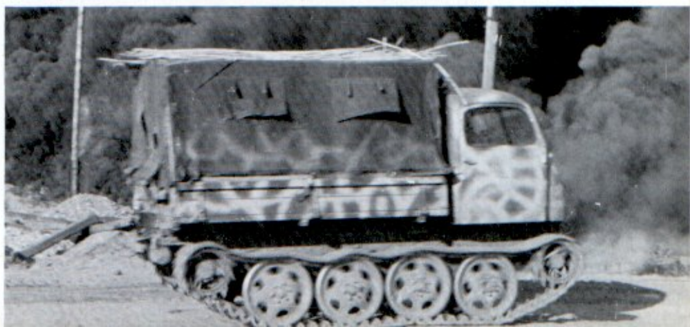
A Steyr RSO tracked truck in Russia. The body and lower part of the cargo bed cover have been oversprayed with connected lines of dark yellow. Long twigs and stalks of hay are carried up on top, probably for additional camouflage from the air. [Bundesarchiv]
