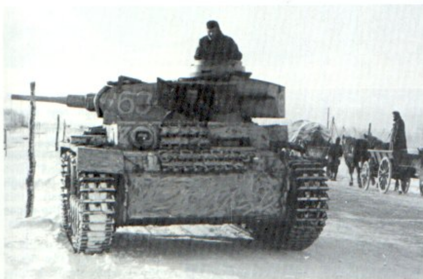
This PzKpfw III ausf G is a good example of the results of paint shortages. The paint has been applied in small strokes to only the front of the hull, and the front and forward sides of the turret. No white paint was applied to any of the rear turret or rear hull surfaces. [Bundesarchiv]
