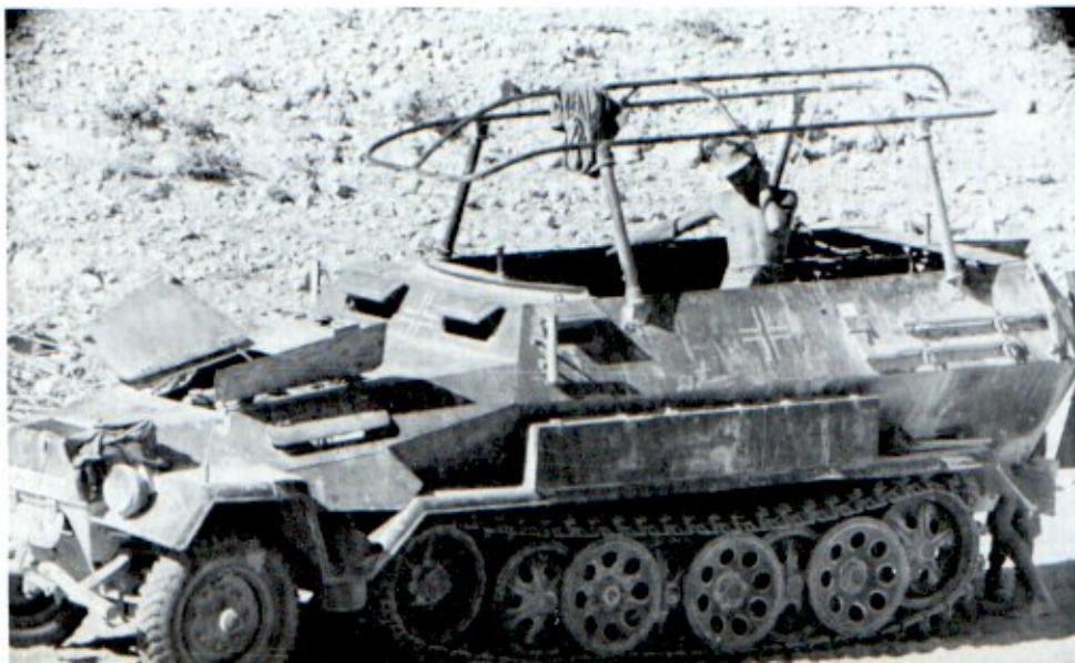
This SdKfz 251/3 ausf B in overall dark gray shows accumulations of dust on upper surfaces and the rear sides of the body. The engine hatches are all open for better ventilation. [Bundesarchiv]
