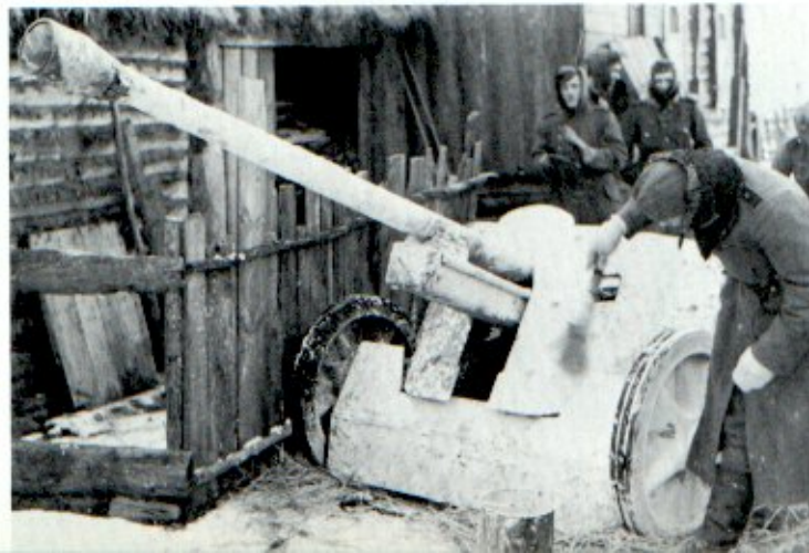
This 5 cm PAK 38 has been splattered all over to make an even coat of whitewash. The paint has built up in globs on the barrel and lower shield. Note the tire is largely covered also. [Bundesarchiv]
