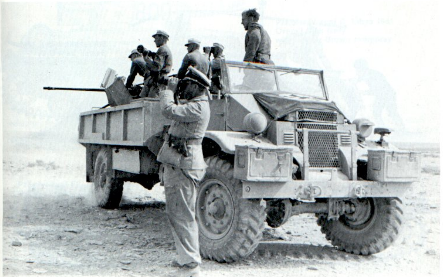
This captured British Canadian CMP truck has been converted into a self-propelled mount for a 2 cm Flak 30. The vehicle, has been repainted in yellow brown overall. The flag is carried to aid in proper identification by Luftwaffe pilots. [Bundesarchiv]
