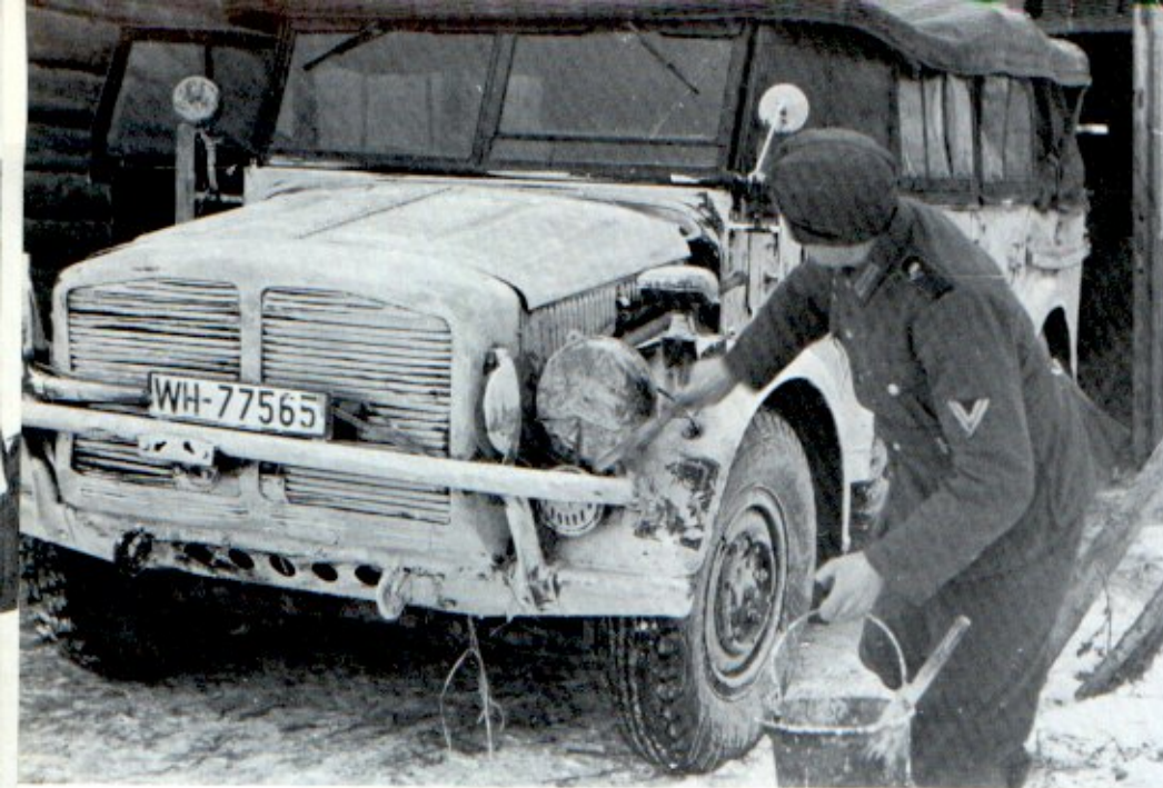
A Horch Kfz 69 s.E.Pkw. at the end of painting in whitewash. The white coating is streaked in spots but has been brushed out to cover the whole body evenly. Here, the top hasn't been painted. [Bundesarchiv]
