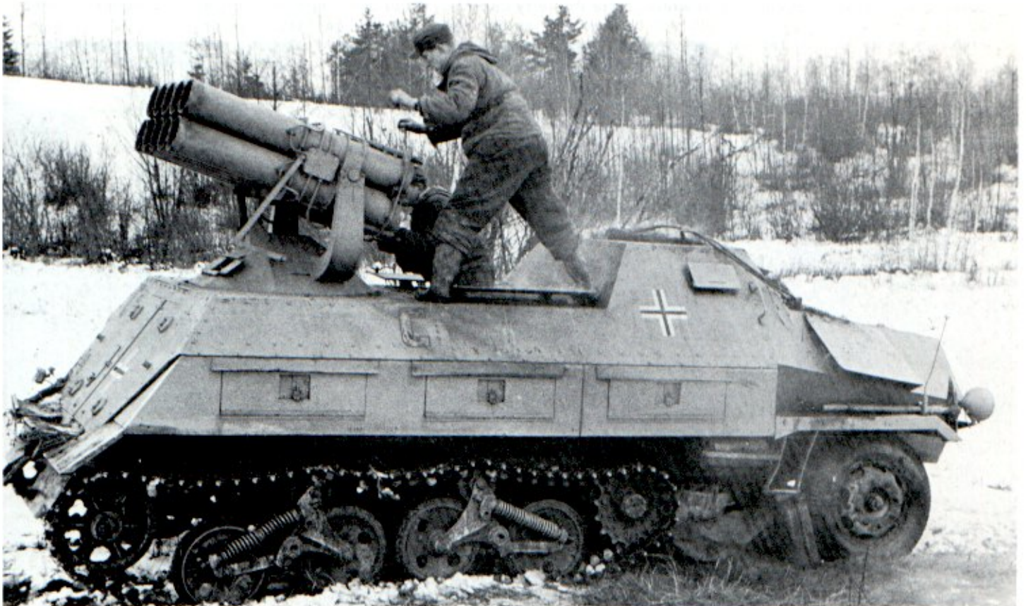
An Opel armored halftrack, Panzerwerfer 42, is seen in Northern Russia in the spring of 1943. The vehicle is painted dark yellow overall. Note the black outline "C" on the side of the halftrack, and the soot streaks from previous firings. The narrow crosses were normally found on these vehicles. [Bundesarchiv]
