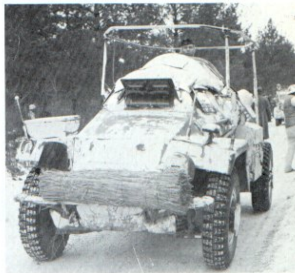
The supplies of white paint and even calcimine whitewash were often limited, and crews had to stretch the amount by painting only parts of the vehicles or by use of patterns of stripes or spots in white. [Bundesarchiv]
