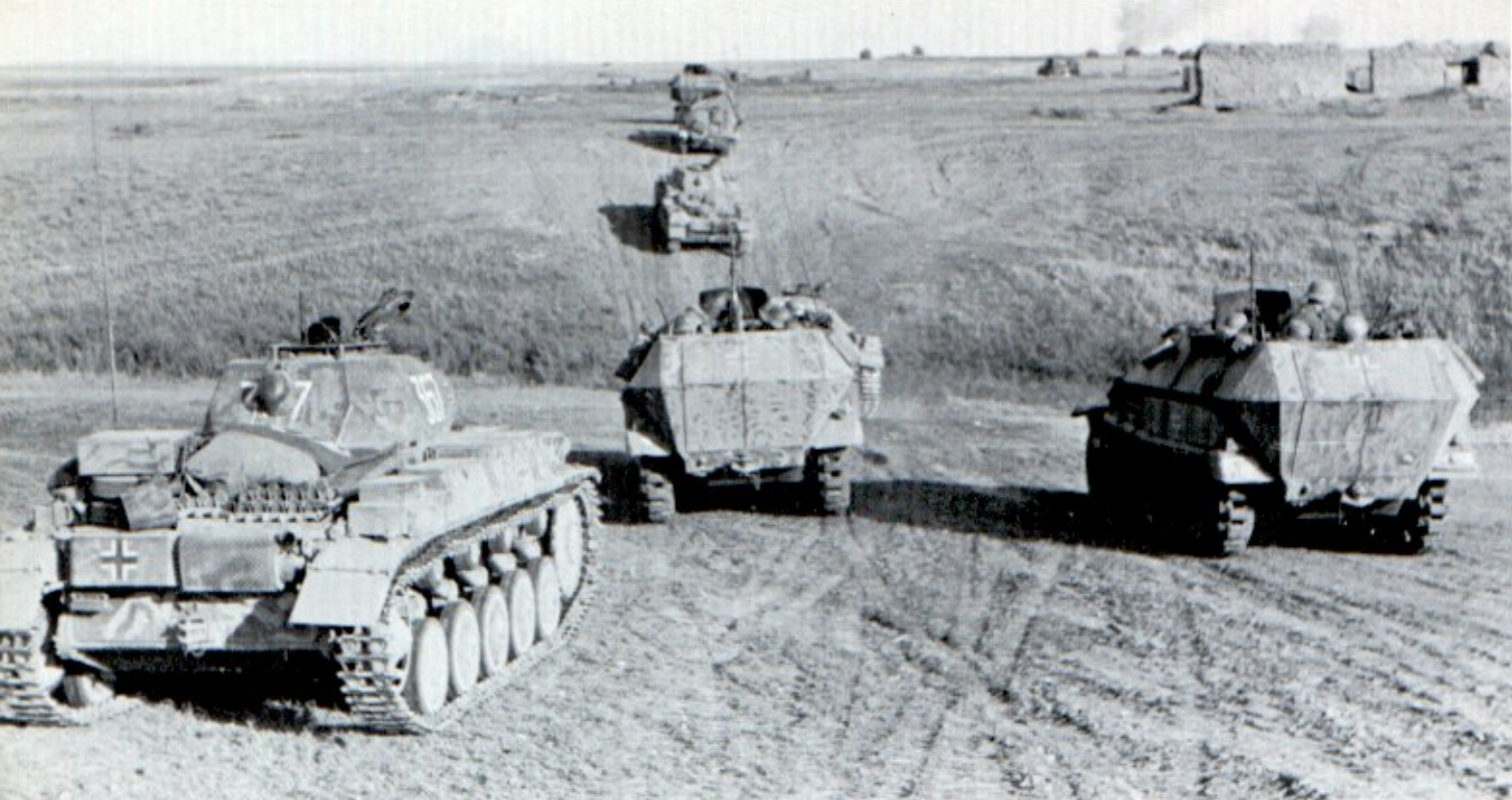
These vehicles show a hastily applied coating of mud, partly brushed and partly smeared in wavy stripes and patches. Dust covering the chassis components has blended with the applied mud and softened it in some areas. [Bundesarchiv]
