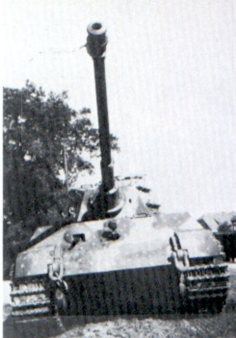
Two different views of a Royal Tiger [Tiger II ausf B] painted in the late war "ambush" scheme. All three colors are used, and the contrasting dark yellow spots on the olive green and red brown show up clearly. Most of the green and red brown spots that are on the dark yellow base have not photographed as well. Note this vehicle has narrow transportation tracks.
