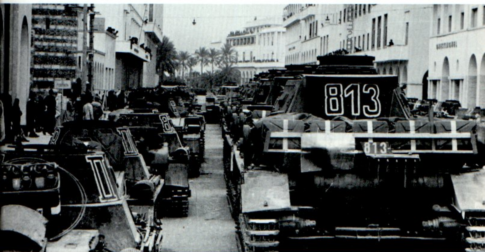
The first armored elements of the embryonic D.A.K. are seen in Tripoli, March 1941. All these vehicles, PzKpfw I's and II's on the left, PzKpfw IV's on the right, are in dark gray. The jerry cans were to be used only for carrying water. Note both large turret numbers in white and the older metal number plate on the rear of the nearest PzKpfw IV ausf D.
