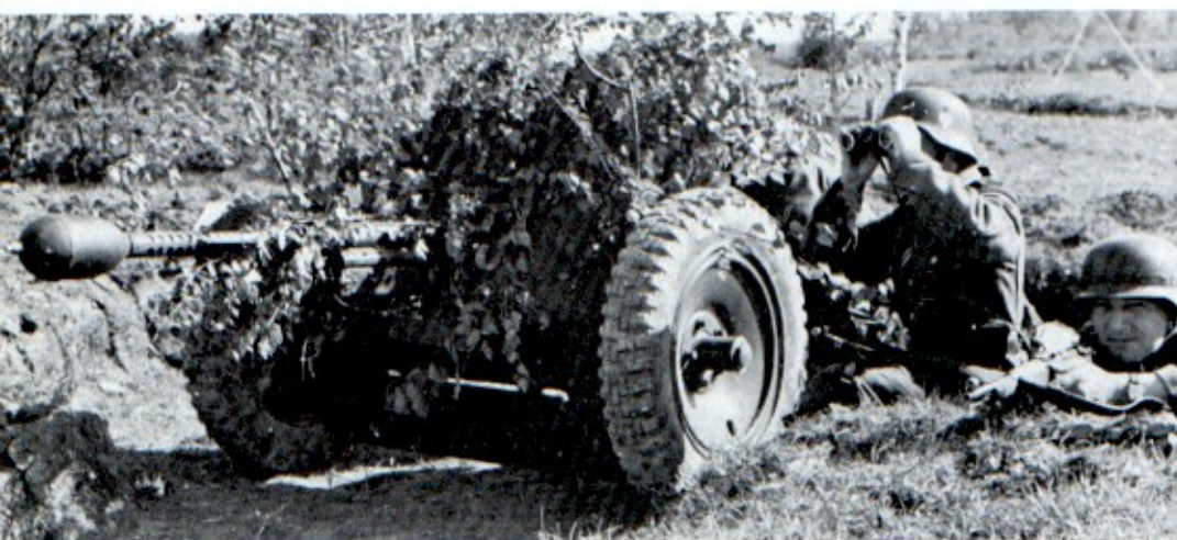
A 3.7 cm PAK 36 with a shaped-charge "Stielgranate" antitank grenade is in dark gray with foliage fastened to the gun and shield to conceal it better from the enemy. [Bundesarchiv]
