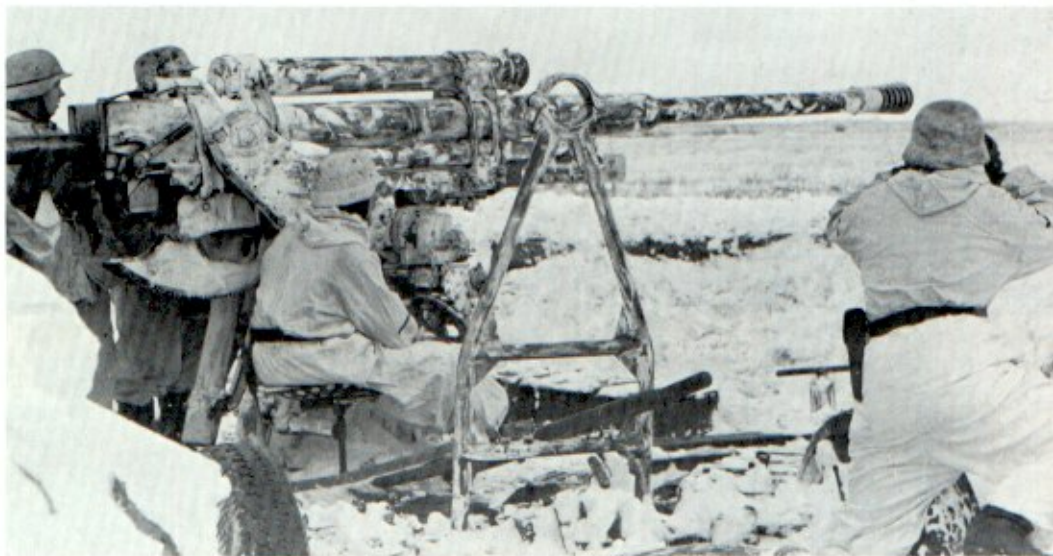
This 7.5 PAK 40 crew has used "natural" camouflage. The grass and straw piled on the gun has held new fallen snow, blending very well with the local fields. This weapon has been emplaced in a ditch to lower the silhouette as much as possible. [Bundesarchiv]
