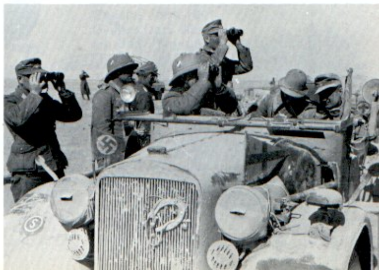
This Horch Kfz 15 has an even coat of mud, which has been worn away from the rear fender by men leaving the car. Scuff marks on other sections expose the dark gray paint. Note the insignia which have been left on a background of dark gray. A wash basin is carried just behind the pennant.
