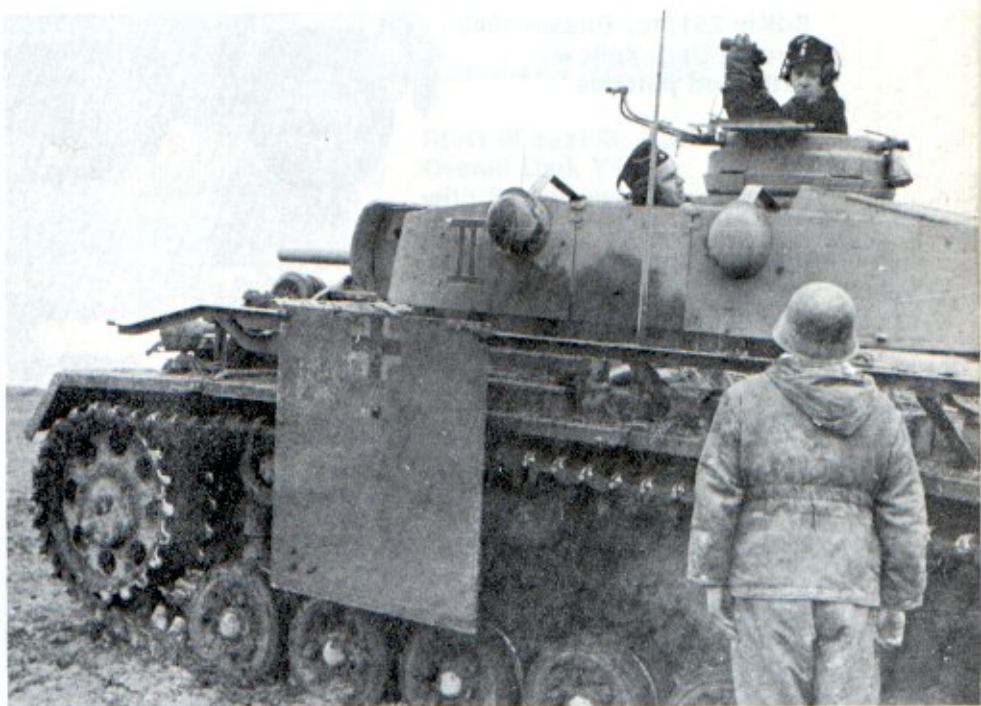
An upgraded early PzKpfw III, possibly an F or G, and used as a command tank, shows the effects of mud being thrown up on the vehicle. The dark areas are wet mud; the lighter areas are dust-covered dark yellow paint. The "II" is in red and white. [Bundesarchiv]
