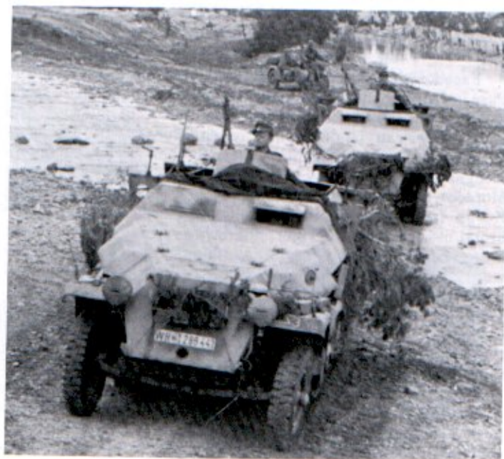
These two SdKfz 251's show different types of repainting. The rear vehicle is overall dark yellow, and may have been a new vehicle, but the front 251 is dark yellow sprayed over the dark gray, some of which shows through. [Bundesarchiv]
