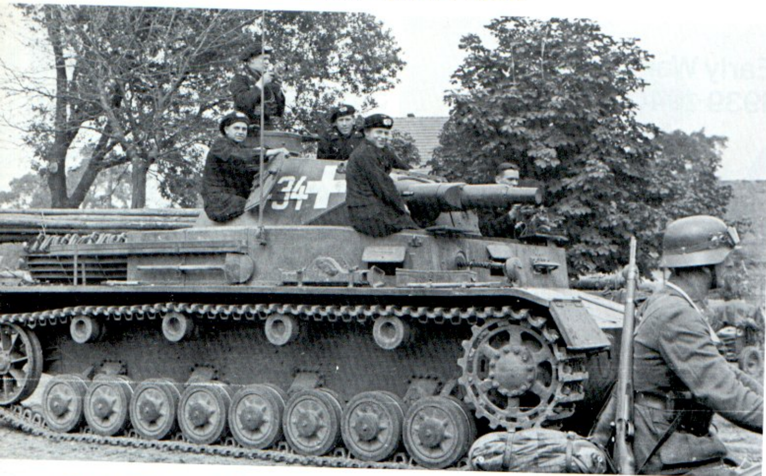
A PzKpfw IV ausf A, seen in Poland, displays the overall dark gray color scheme used by most German armored vehicles at this time. The turret numbers and solid cross are in white. Note the spare tracks above the antenna trough, and the saplings logs on the rear deck. [Bundesarchiv]
