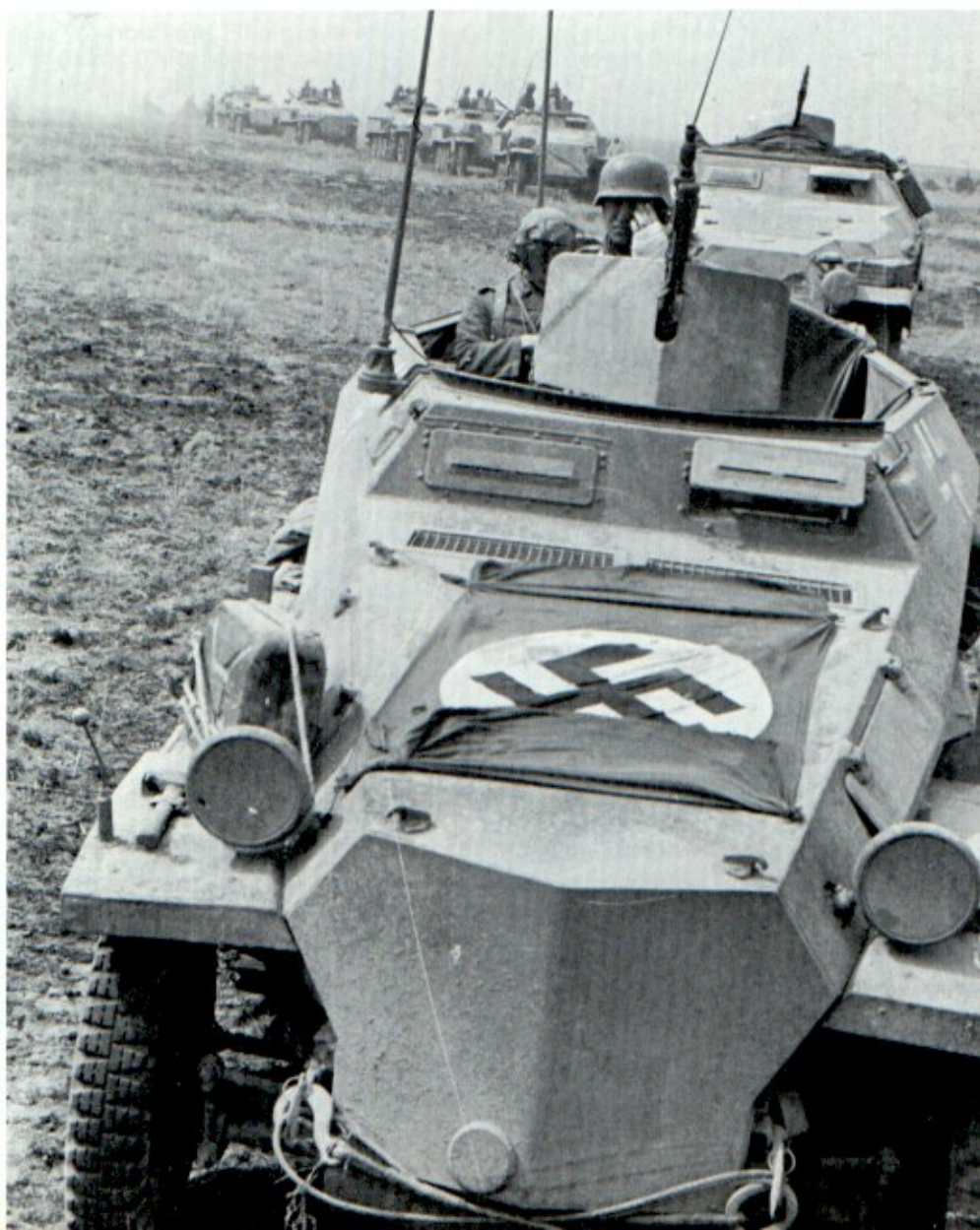
These halftracks, photographed in the summer of 1942, are in overall dark gray, but a heavy layer of sprayed and splattered mud and dust hides the gray almost completely. The lead vehicle is a SdKfz 250/3 radio vehicle. [Bundesarchiv]
