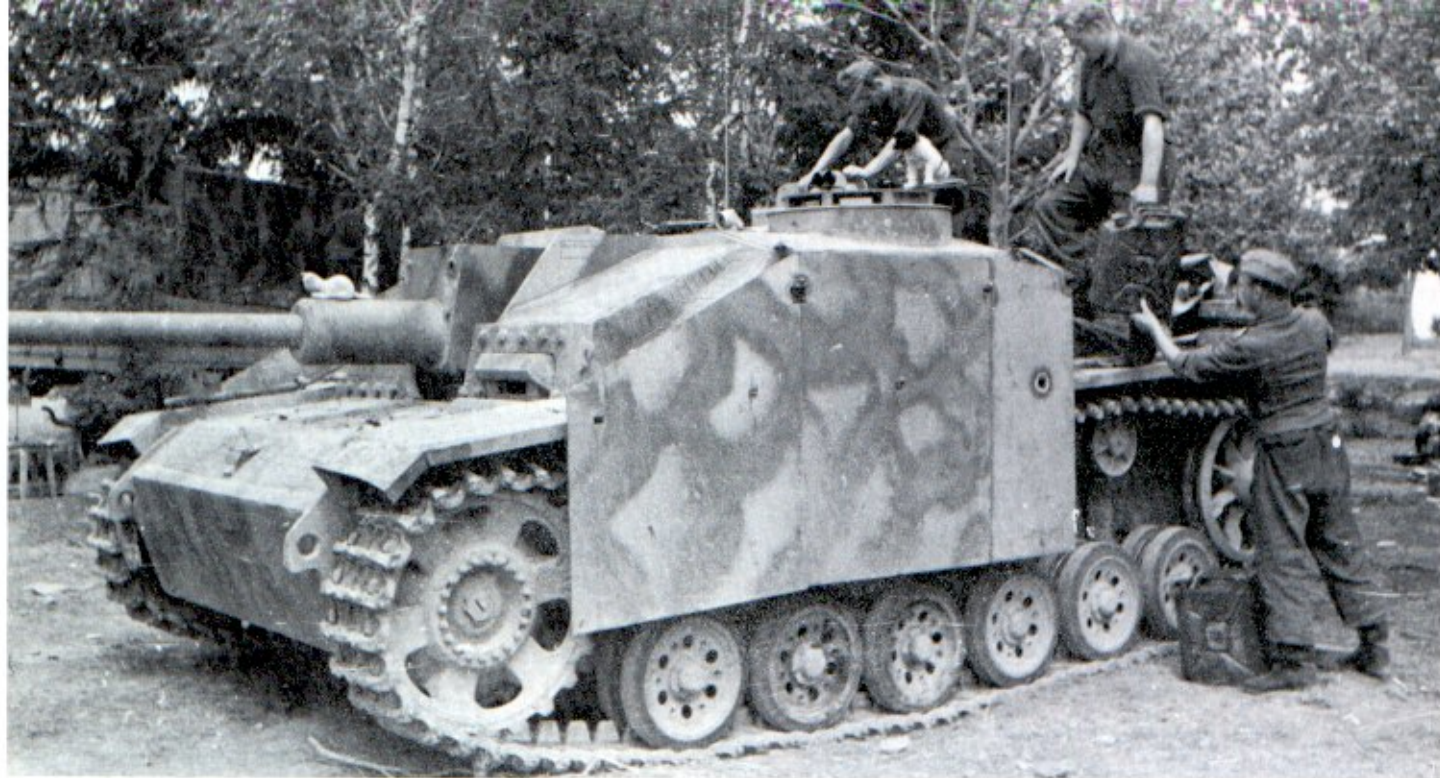
This StuG III ausf G has a scheme found often in southern Russia and Rumania. Base color is dark yellow. Red brown is sprayed in connected patches with olive green outlines. [Bundesarchiv]
