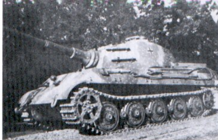
Two different views of a Royal Tiger [Tiger II ausf B] painted in the late war "ambush" scheme. All three colors are used, and the contrasting dark yellow spots on the olive green and red brown show up clearly. Most of the green and red brown spots that are on the dark yellow base have not photographed as well. Note this vehicle has narrow transportation tracks.
