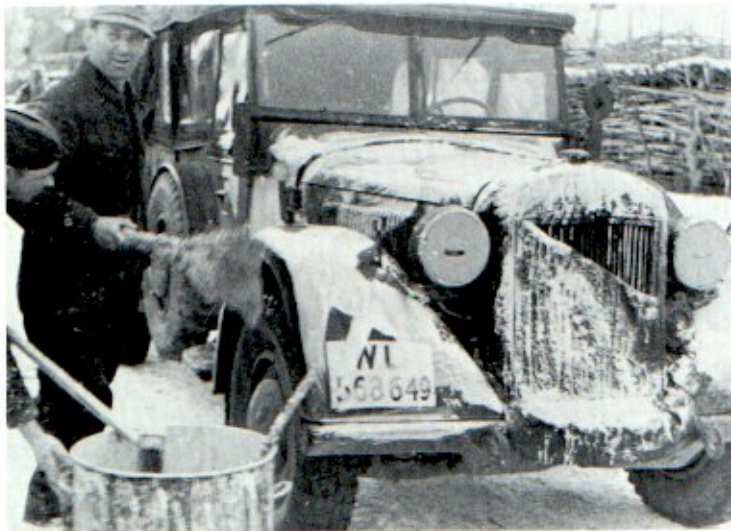
A Horch Kfz 15 m.E.Pkw receives a rough coat of whitewash, applied with a small push broom, and a straw broom used to splatter the whitewash all over the vehicle. The push broom was used to smooth out the splattered coating and give an overall white finish. [Bundesarchiv]
