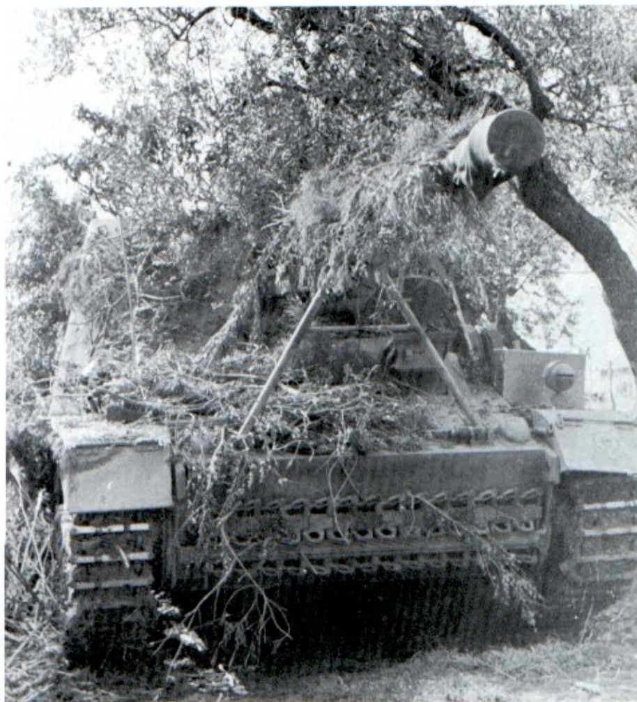
A "Hummel" parked in a roadside shelter. Foliage breaks up the vehicles shape and extra branches have been laid around the chassis to hide the wheels. Colors are dark yellow and light sprays of olive green. [Bundesarchiv]
