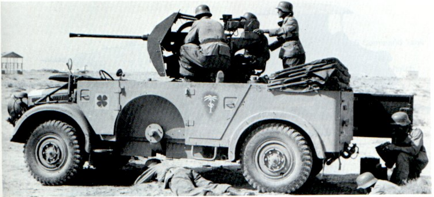
This Horch s.E. Pkw, Kfz 69, has been converted into a self-propelled mount for the 2 cm Flak 38. The yellow brown has been sprayed neatly over the entire vehicle, with a small area of original dark gray showing around the Afrika palm. The Flak 38 is still in dark gray. The four-leaf clover is green on a white square. [Bundesarchiv]
