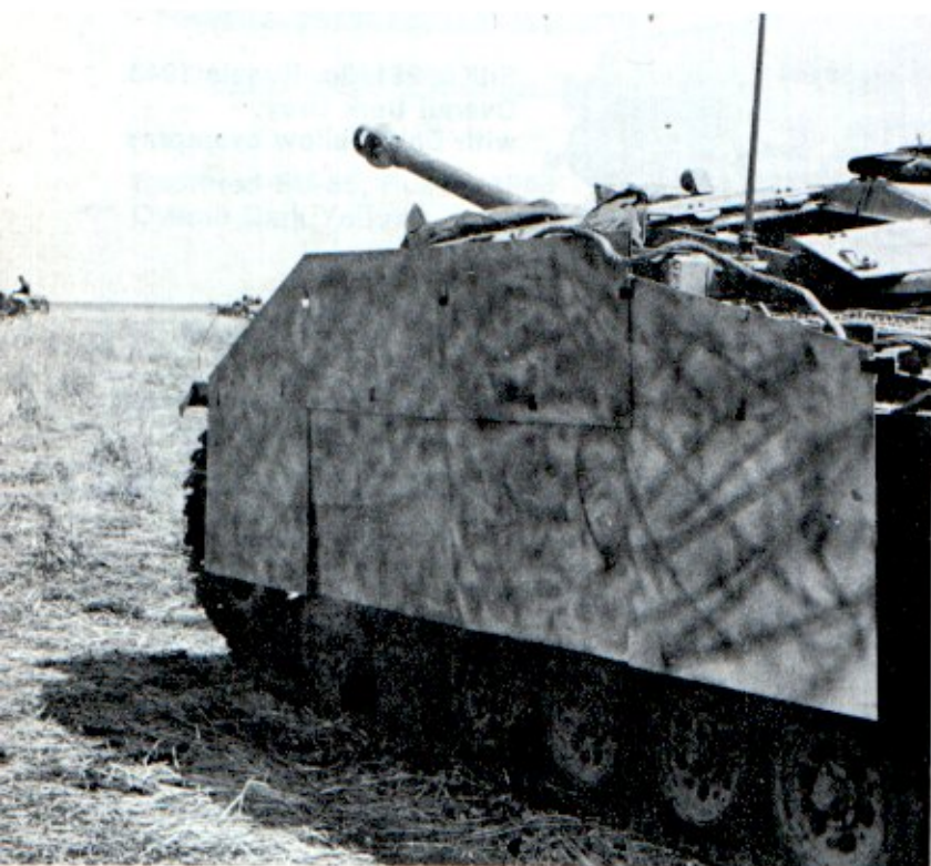
This StuG III ausf F in Russia is painted dark yellow. A very fast and rough pattern of sprayed strokes in olive green has been applied to the skirts. Very little time was allotted to this job. [Bundesarchiv]
