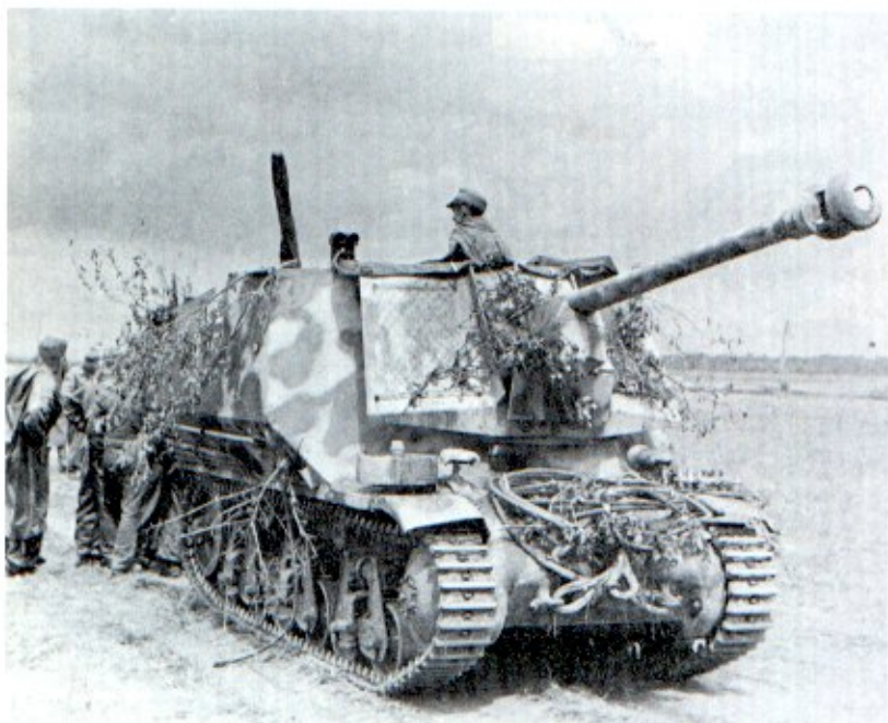
A "Marder I", built on a Hotchkiss H35 chassis, has red brown and dark olive green sprayed over dark yellow. Note the use of chain link fencing to attach extra foliage. [Bundesarchiv]
