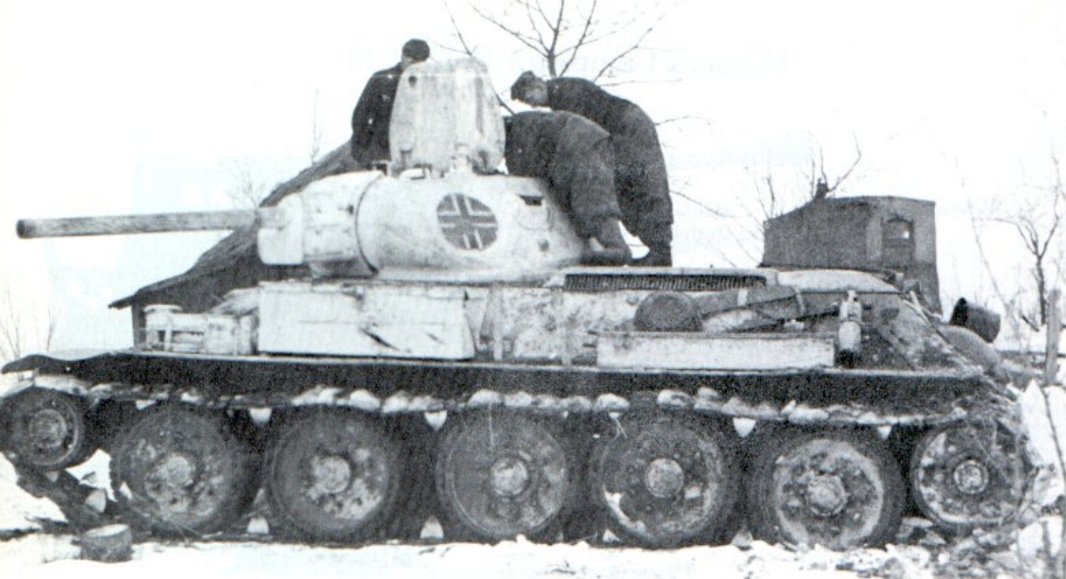
A T34/76 model 42 in a solid coat of white paint. The rear of the hull and the chassis have not been painted, and the insignia on the turret is in a circle of dark gray color left in the painting with white. [Bundesarchiv]
