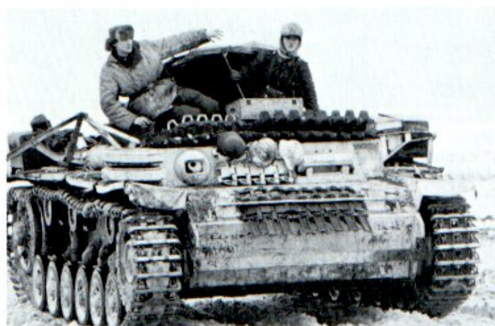
An old PzKpfw III, now used as an ammunition carrier, carries a scruffy but complete coat of white paint. The turret ring is covered by the round tarpaulin, and a great deal of extra tracks and fittings are stowed on the vehicle. The tracks on the bow are "ostketten", the wide tracks designed for use in the poor weather and rough terrain of the Russian front. [Bundesarchiv]
