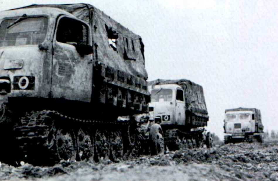
These Steyr Raupenschlepper Ost [RSO] trucks move through thick mud. Their white camouflage paint is wearing off. Many crews didn't remove the paint, but just stopped touching up the defects, and let it wear off gradually. [Bundesarchiv]
