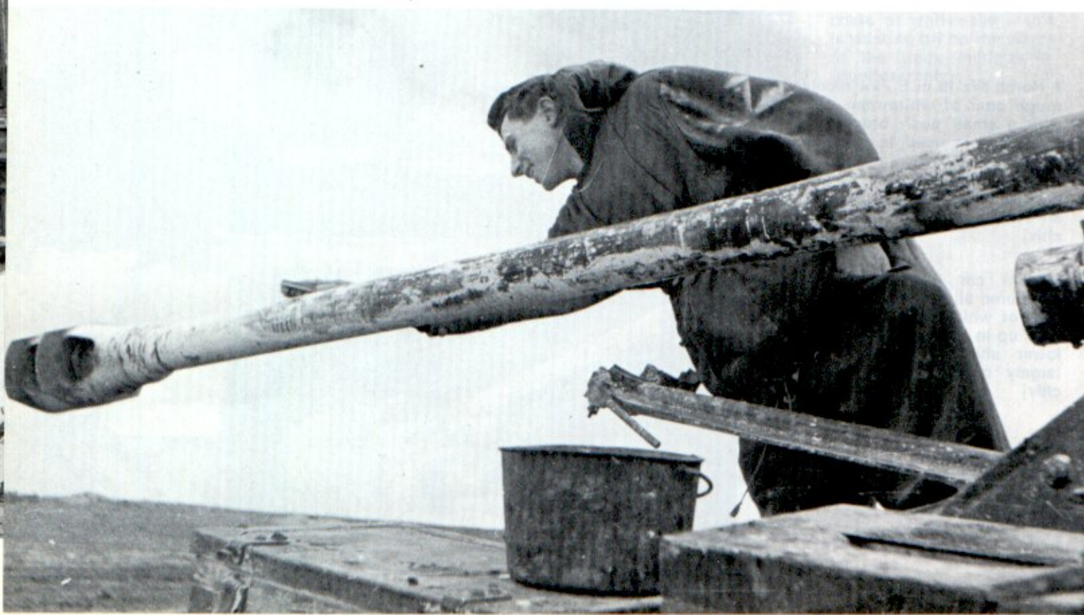
This crewman of a "Rhinoceros" self-propelled 8.8 cm gun is washing off the white winter camouflage paint. Both the paint and whitewash were removed with water. [Bundesarchiv]
