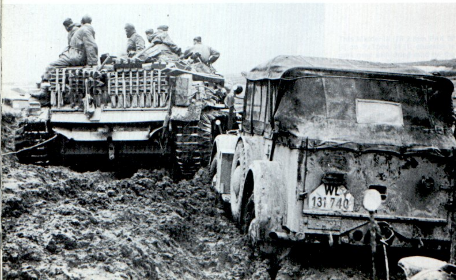
A StuG III ausf F and a Horch Kfz 15 plow through the mud of spring, 1943. The Horch is still overall dark gray, with an even layer of dust - further covered by freshly deposited mud. Note the "ostketten" in use on the StuG III and stowed on the rear.
