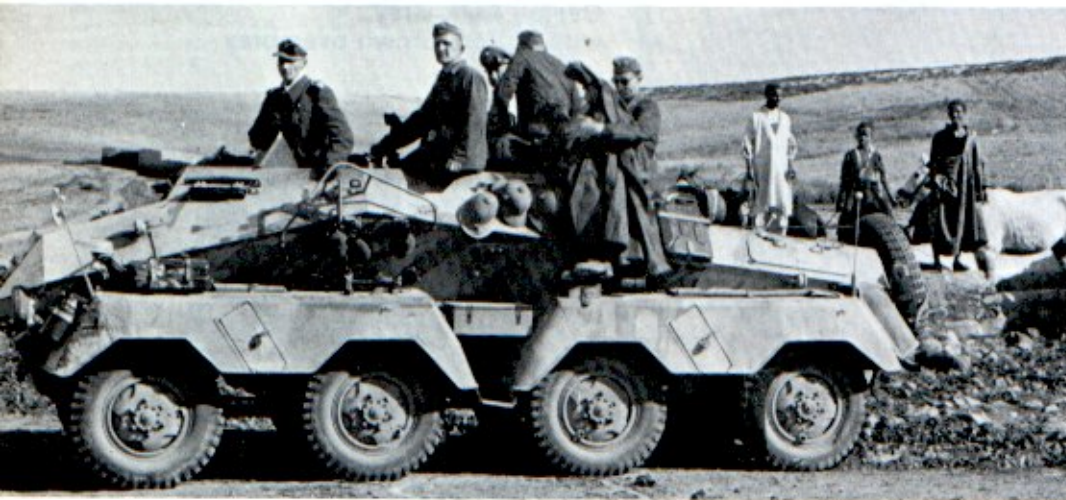
A SdKfz 233 self-propelled 7.5 cm howitzer, also seen in Tunisia. The desert brown paint is somewhat streaked and weathered. Note the old style pith helmets still carried. [Bundesarchiv]
