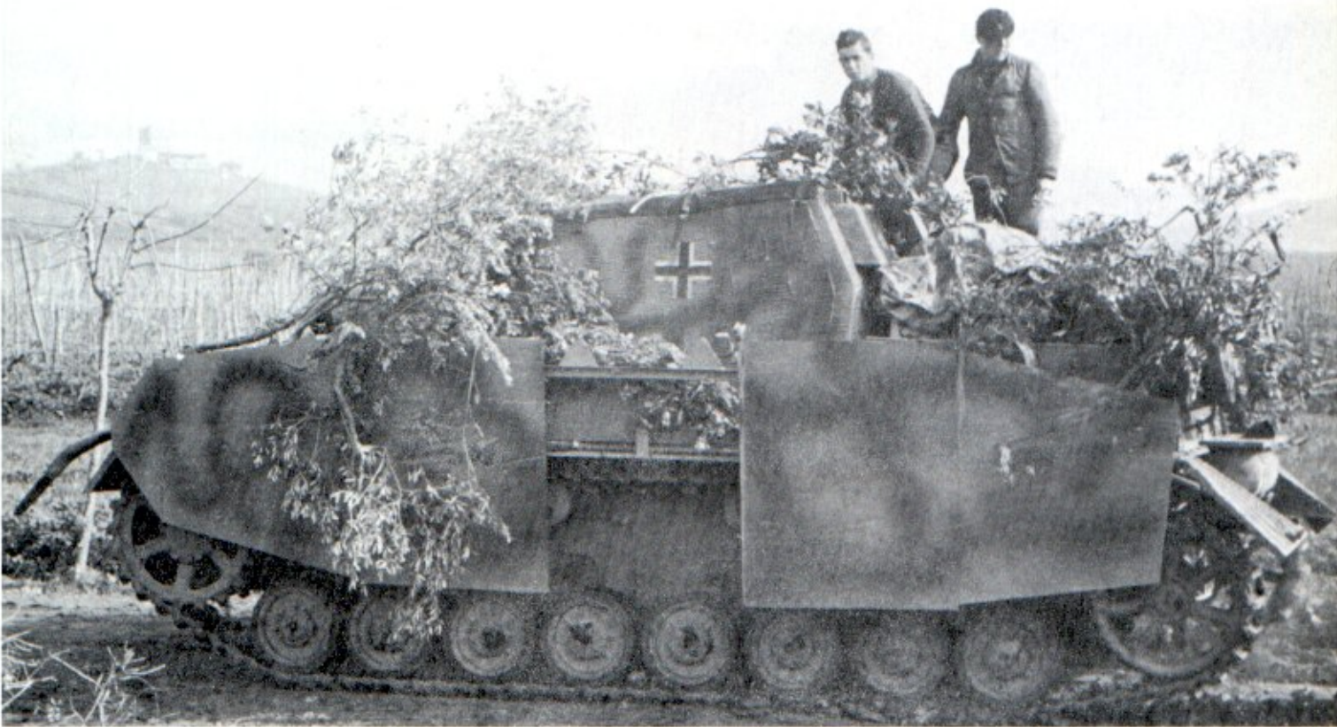
A Sturmpanzer IV "Grizzly Bear" photographed in Italy in 1944. Colors are dark yellow with red brown sprayed lines. Foliage has been piled on top of the front and rear to conceal the square shapes of the superstructure. [Bundesarchiv]
