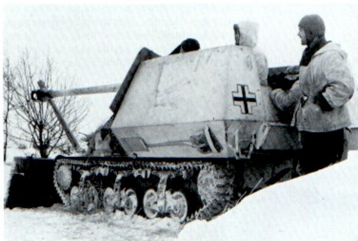
A Marder I [PAK 40 on the French "Lorraine" chassis] seen in a very even application of white paint. Packed snow provides additional camouflage on the wheels and tracks [Bundesarchiv]
